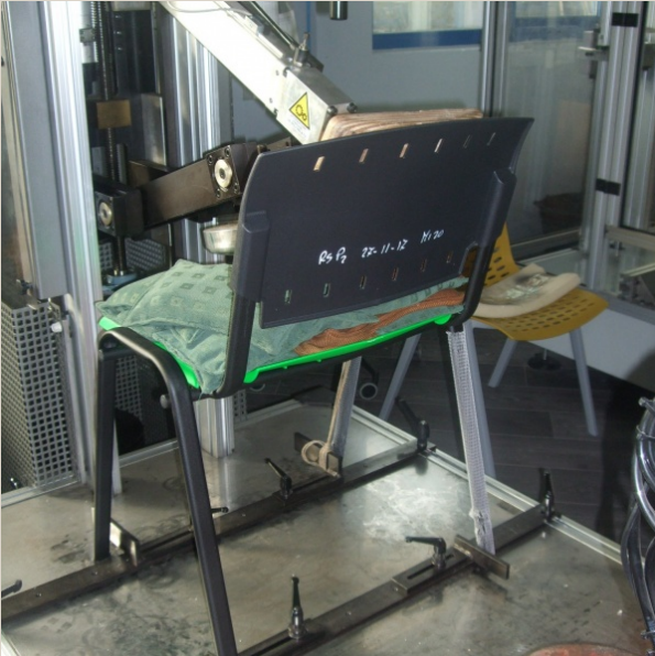
Static load test
